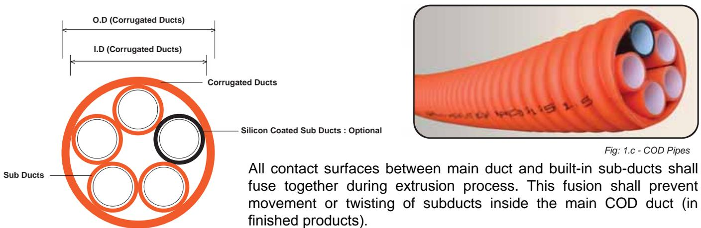
All contact surfaces between main duct and built-in sub-ducts shall fuse together during extrusion process. This fusion shall prevent movement or twisting of subducts inside the main COD duct (in finished products).
